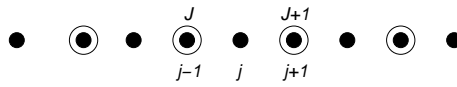
Figure 14: Illustration of coarse and fine meshes in one dimension for the purpose of linear interpolation (prolongation), of coarse grid values to the fine grid. Refer to the text for details.
