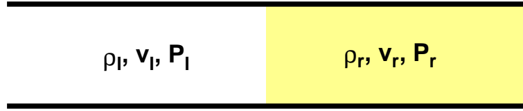
Figure 2.2: A schematic diagram of a fluid shock tube's initial configuration. A divider separates two independently prepared fluid states. The divider is removed at t = 0 , and the Riemann initial value problem allows one to determine the subsequent evolution.
