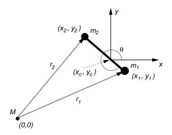
Consider two test masses,  $m_1$ ,  $m_2$  connected by a massless rigid rod of length d, in orbit about a mass,  $M \gg m_1, m_2$  as shown in the figure above. Let  $(x_i, y_i), i = 1, 2$  be the coordinates of the two test masses, let  $(x_c, y_c)$  be the coordinates of the dumbbell's center of mass, and let  $\theta$  be the angle the rod makes with the x-axis. Defining
